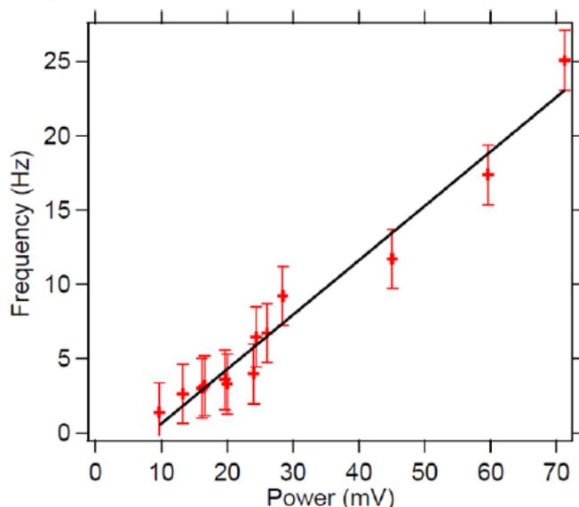
Fig. 1: The rotation rate of a birefringent particle goes to zero close to a hydrophilic (regular glass slide) surface at non-zero laser powers due to binding.
